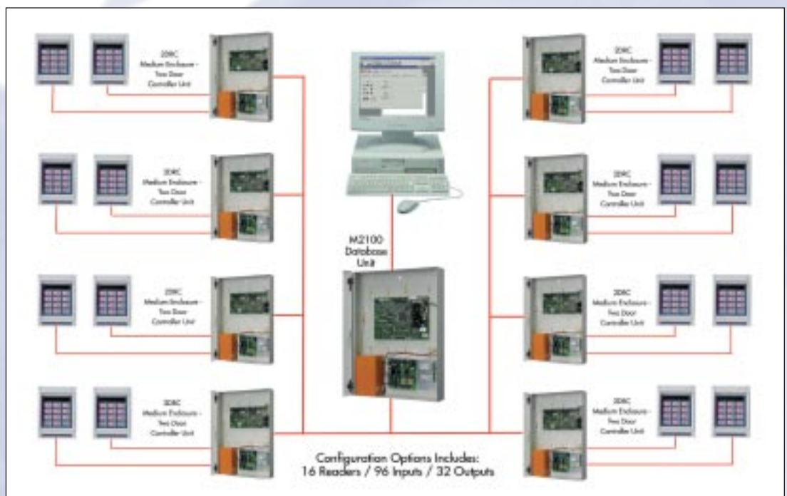
Maximum 16 reader configuration using DBU and eight 2DCR's
